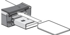
Remove the cap from the end of the modem and insert the USIM card into the top slot, as shown in the illustration. Push the USIM card in until it clicks into place. To remove it, push it in and then release it.
