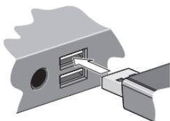
Insert the C01SW modem into the USB slot.
