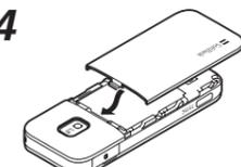
**4** Slide Battery Cover into 731SC Slots; replace Battery Cover
