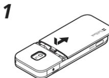
**1** Press down to slide Battery Cover loose
