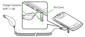
2 Insert Charger Connector into lighter socket
