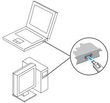
After executing "Stop Hardware Device," LED Status Lamp may light or flash. This is normal. Remove modem from PC.
