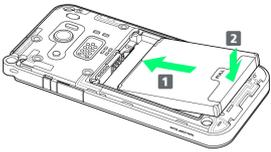
· Slide Battery into place as shown.
