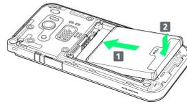
· Slide Battery into place as shown.
