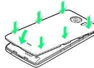
· Align External Connector Port sides, then press down firmly along edges.
